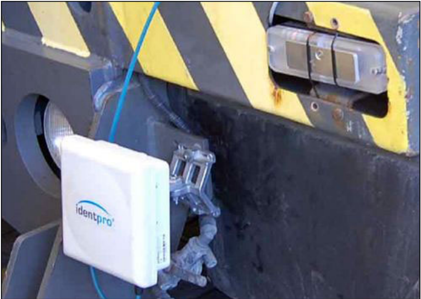
The tug vehicle's rear bumper is equipped with a Deister RFID reader (upper right) and a reader antenna (lower left).
